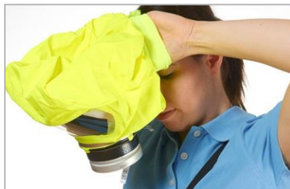
Widen the neck seal and pull the hood over your head. The inner head harness automatically adjusts to your head. Ensure that nose and chin sit comfortably in the half mask and that all hair is tucked into the hood.
