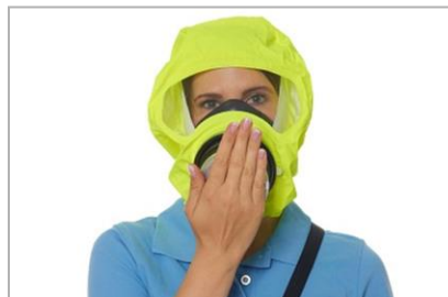
Check the fit of the half mask by closing the front filtering opening with the palm of your hand. If negative pressure is not generated readjust the half mask to ensure a close fit over nose and mouth.
